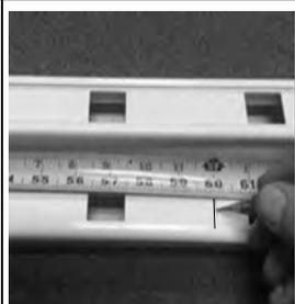
9. Now mark the Top Rail (A) 3/8" shorter on each end than the Bottom Rail (B) was marked also ensuring the baluster holes are centered. Cut to length the Top Rail (A) and Bottom Rail (B) along the marked lines.
