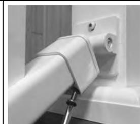
17. Apply Adhesive Tab (M) to flat, top surface of the Top Rail (A), near the post. Slide Bracket Covers (F) to interlock with flange on the Saddle Brackets (E).
