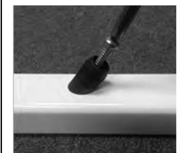
11. To assemble rail, begin with Top Rail (A) and insert balusters into each baluster hole. Use a rubber mallet to tap the balusters into place until fully seated into the Top Rail.
