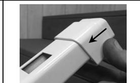
15. At the point(s) where you installed Support Block Connector(s) (step 11), carefully measure the distance from the underside of the bottom rail (B) to the floor or step. Cut support block material (H) to fit. Slip the Support Block(s) over Support Block Connector(s) (I). Slide the rail back into place and make certain the rail is plumb.
