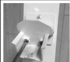
7. Align the Bottom Rail Hinge Assemblies (D) so they are facing parallel to each other, and measure the distance between upper and lower Bottom Rail Hinge Assemblies (D) previously mounted on the posts in step 5.
